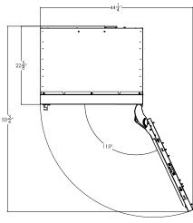
Max clearance required for opened door is 49-3/4" when opened to 90°\* (dimensions shown are without door overlay installed.)
