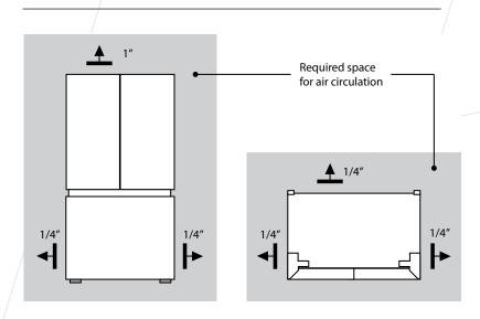
The refrigerator should be placed in a dry, well-ventilated area with a minimum of 1/4" clearance at back and sides and 1" clearance above.
