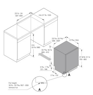
$\mbox{\ensuremath{\,\star}}$  Flexible side trims (width without side trims: 23  $\ensuremath{\,\%_{16}}$  / 596)
