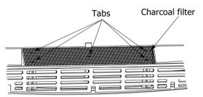
Reinstall the vent by sliding the bottom of the vent into place. Push the vent top into position and slide right into place. Replace the two vent mounting screws located on top of the microwave using a #1Phillips screwdriver.
