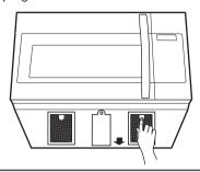
2. To remove grease filters, Pull filters latch downward. The filter will drop out.
