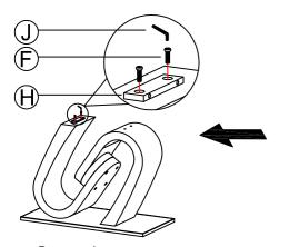
Remove the upper and lower shipping block from the pedestal
