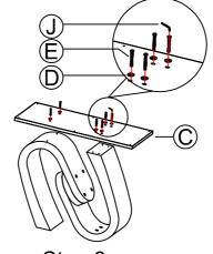
Step 3 Attach the bottom plate to the pedestal
