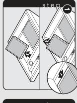
Slide filter front over front lip. Push filter rear up, then slide back over rear lip.
