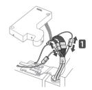
3 Rotate the hinge lever counterclockwise 1. Lift the top hinge 2 free of the hinge lever latch.
