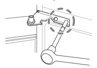
2 Twist the hinge to raise the pivoting end so that the door can be lifted off.
