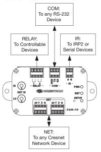
**CAUTION**: Incorrect wiring may damage the C2N-IO.
