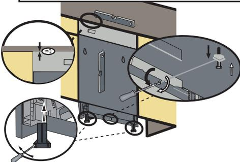
If the height of the enclosure is above 34 9/32" (870mm) use long supports as shown in the figure.
