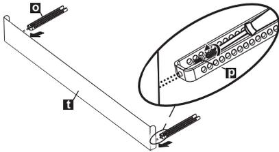
1. A. If the height is 32 9/32" to 34 9/32" (820mm-870mm) and use short supports; adjustable plinth metal with 80 mm length (v), toe kick brackets(o) are installed. Mounting is done using Screws  $\varnothing$  5/32" x 7/32" ( $\varnothing$  4mm x 6mm) with a Philips Screwdriver.
