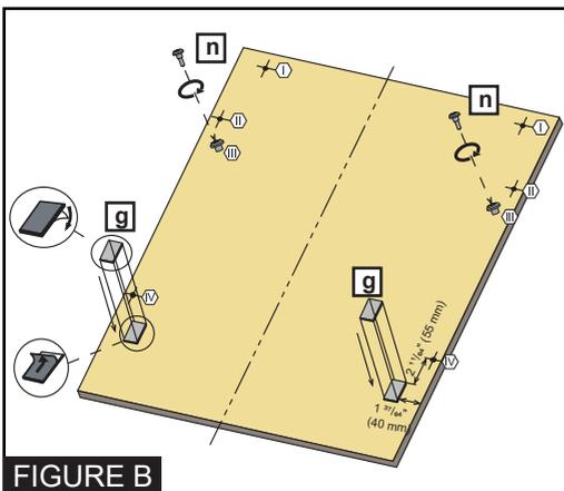
3- As shown in Figure B, Screws  $\varnothing 5/32" \times 27/32"$  ( $\varnothing 4\text{mm} \times 21,5\text{mm}$ ) is installed in positions III.
