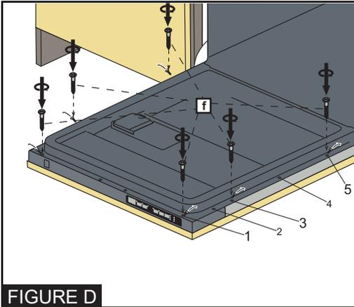
7- As shown in Figure D, Screws  $\text{Ø } 5/32'' \times 53/32''$  ( $\text{Ø } 4\text{mm} \times 42,5\text{mm}$ ) are installed in positions I, III and V.
