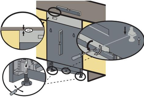
If the height of the enclosure is 32 9/32" to 34 9/32" (820mm-870mm) use short supports as shown in the figure.
