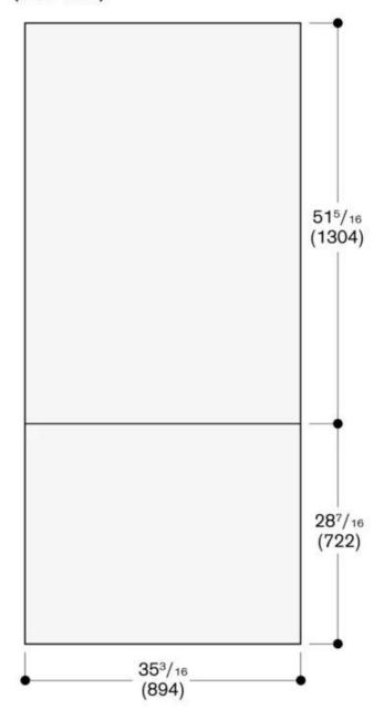
The door panel thickness is 3/4" (19 mm)
