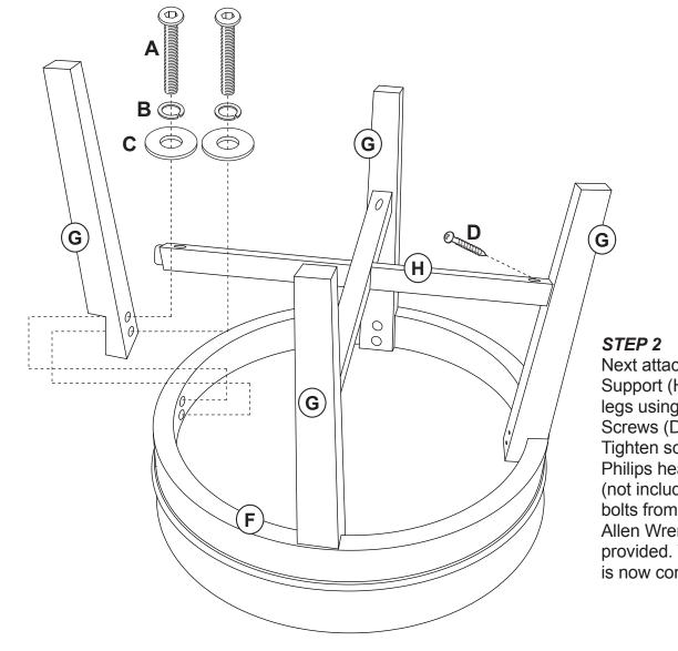
Next attach Cross Support (H) in between legs using 2 Wood Screws (D) per stretcher. Tighten screws with Philips head screwdriver (not included). Tighten all bolts from step 1 with Allen Wrench (E) provided. The assembly is now complete.
