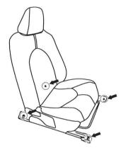
10 Tilt the passenger seat towards the back to reveal (2) connectors. Disconnect and remove the seat.
