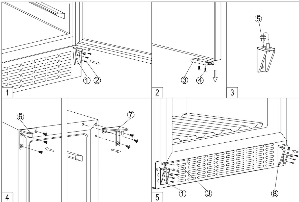
1. Remove the bottom hinge 1 by unscrewing the four lock screws 2. Be careful to hold the glass door firmly after removing the screws. (Fig. 1)
