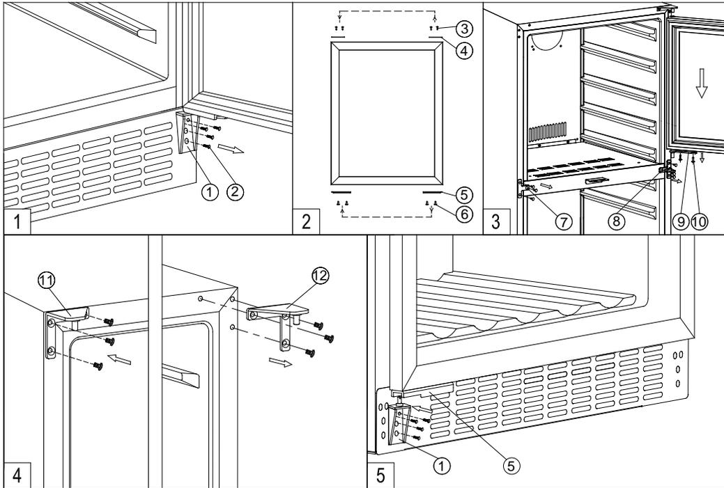
1. Remove the bottom hinge **1** by unscrewing the four lock screws **2**. Be careful to hold the lower glass door firmly after removing the screws. Then gently pull down to remove the lower glass door from the middle hinge **8** and place it on a padded surface to avoid the risk of damage. (Fig. 1)
