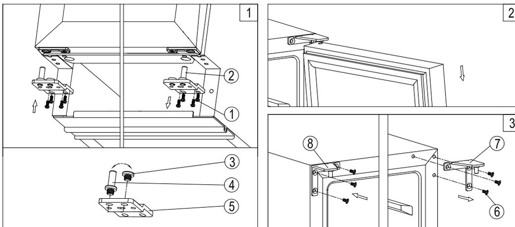
1. Remove the bottom hinge **2** by unscrewing the four lock screws **1**. Be careful to hold the door firmly after removing the screws. (Fig. 1)
