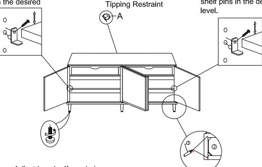
Adjust Leveler if needed to level case on uneven floor.
