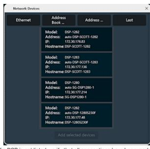
NOTE: If a DSP is not listed, verify that all connections have been made and that all devices and the computer running the Crestron Avia Audio tool are on the
