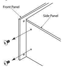
2. Secure the rack mounting bracket to the MIP200 side panel using 2 of the 8-32 thread (larger) flathead screws. Do not re-use the previously removed screws. Use 2 of the supplied 6-32 thread (smaller) flathead screws to secure the bracket to the front panel.
