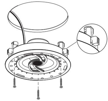
Center the speaker in the cutout. Rotate the frame as needed before tightening the screws. Tighten the screws equally until the clamps secure the frame.
