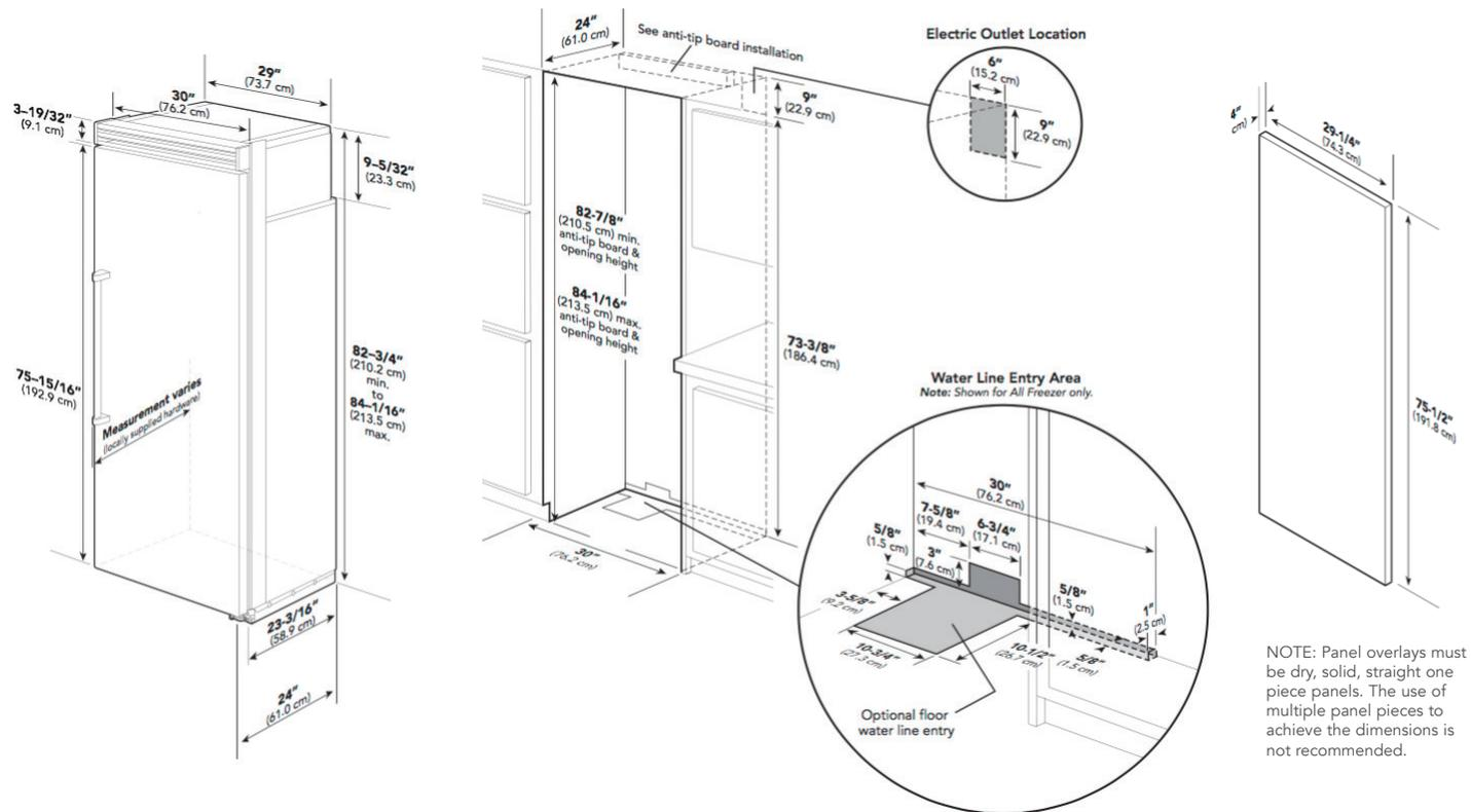
\*Custom panel models fit flush in 25" (63.5 cm) deep cabinet openings. They can be installed in standard 24" (61.0 cm) deep openings. The door faces and top grille will protrude 3/4" (1.9 cm) into the room.
