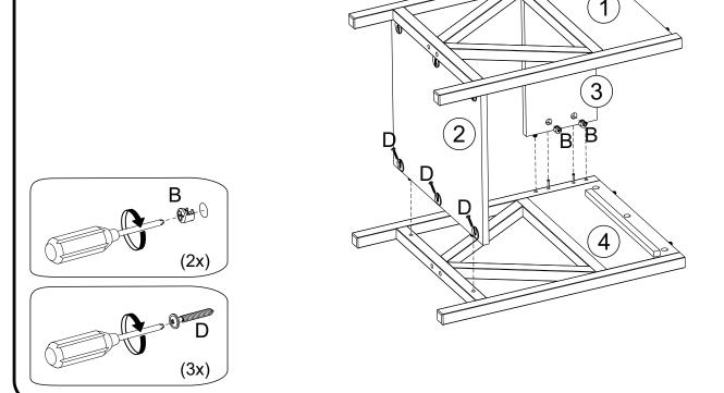
$Step \ 5 \ \ ^{\text{Attach the body to part 5 using Cam Locks (B)}}.$
