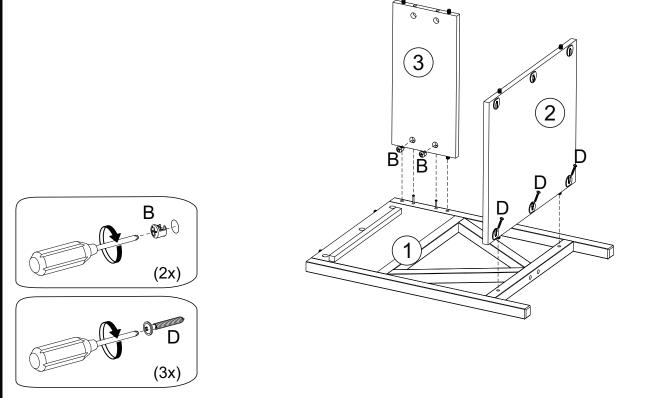
Step 4 Attach parts 1, 2, 3 to part 4 using Screw (D) and Cam Locks (B).
