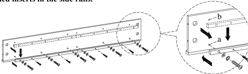
**STEP 6:** Screw the bolts (E) into HB & FB. Make sure the slat bearer is in the LOWER position. Align the bolts with the holes in the end of side rails and attach the side rails to HB & FB using half moon washers (F) and nuts (G). Then use a hex wrench (H) to tighten all the nuts.
