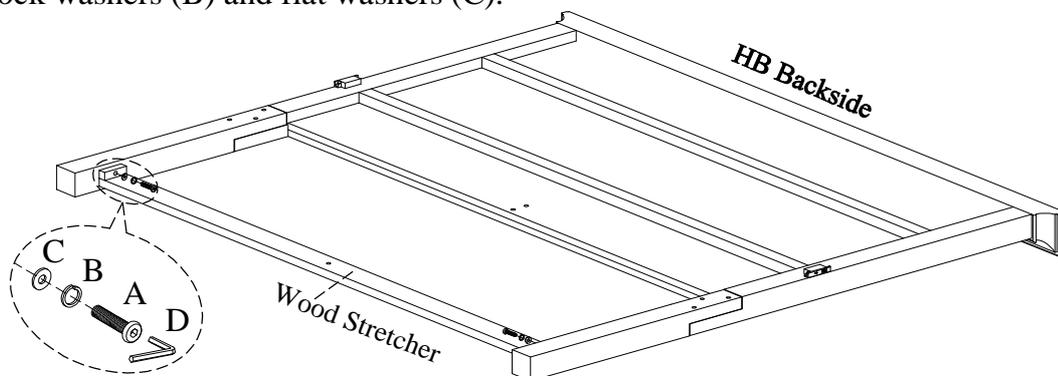
**STEP 3:** Attach the center support leg to headboard and wood stretcher by using 3 bolts (A), lock washers (B) and flat washers (C). Completely tighten all bolts.
