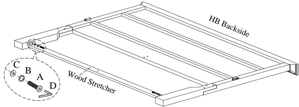
**STEP 3:** Attach the center support leg to headboard and wood stretcher by using 3 bolts (A), lock washers (B) and flat washers (C). Completely tighten all bolts.
