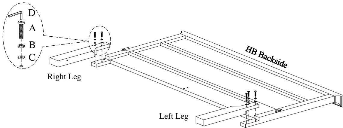
**STEP 2:** Attach the wood stretcher to the legs by using 2 bolts (A), lock washers (B) and flat washers (C).
