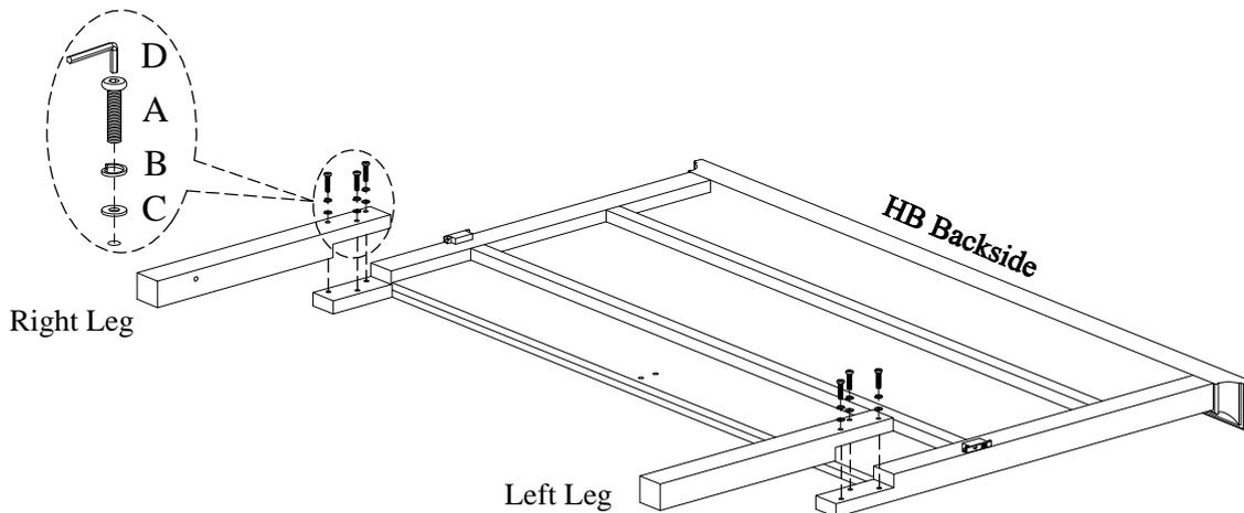
**STEP 2:** Attach the wood stretcher to the legs by using 2 bolts (A), lock washers (B) and flat washers (C).
