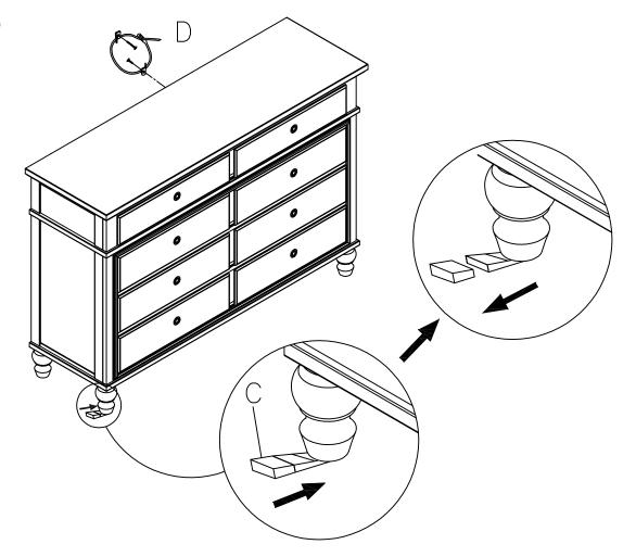
NOTE: IF THE UNIT IS PLACED ON AN UNLEVEL SURFACE, PLACE A LEVELER UNDERNEATH ONE FOOT UNTIL THE UNIT IS LEVEL. BREAK OFF ANY PROTRUDING SEGMENTS.
