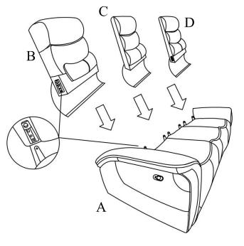
Step 2: Attach the LSF (E) and RSF(F) Wing to Backrest (B & D).
