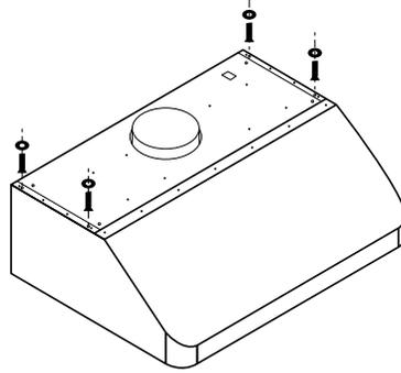
3. Secure the recirculating kit with the provided screws. Once secure, begin tightening each screw until the recirculating kit is flush with the range hood.
