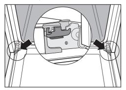
The door is connected with brackets on each door hinge.
