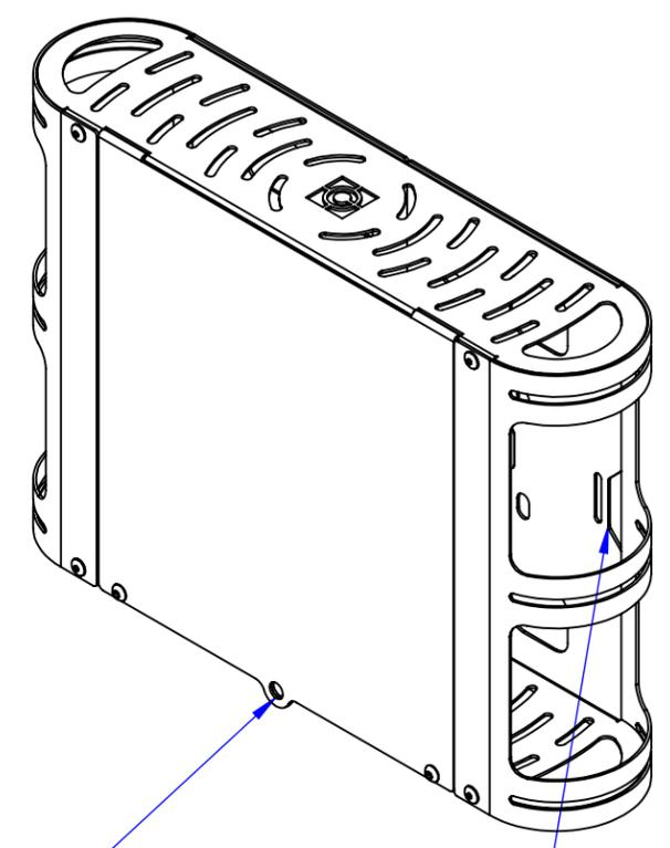
SECURITY HOLE FOR 5/16" DIAMETER PAD LOCK
