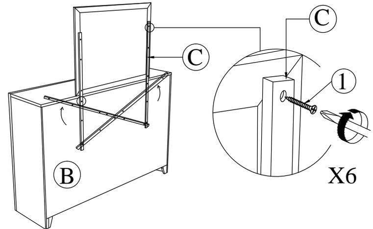
**STEP 3 :** Tighten the Flat Head Chipboard Screw ( 1 ) as shown.
