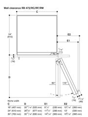
The drawing is based on a cabinet panel width of  $^3/_4$ " (19 mm) and a Gaggenau cabinet handle height of  $1^5/_{16}$ " (49 mm).
