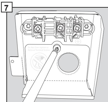
Remove strain relief plate. **Do not discard!** This will be reinstalled later.
