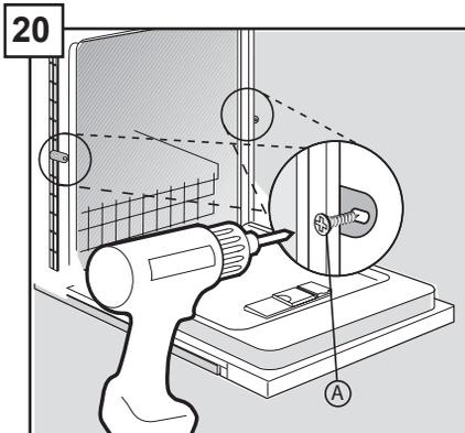
Insert screws (Part A) through pre-positioned mounting brackets on each side of the unit and attach to enclosure (pre-drilling of holes recommended). Remove upper rack before inserting screws.
