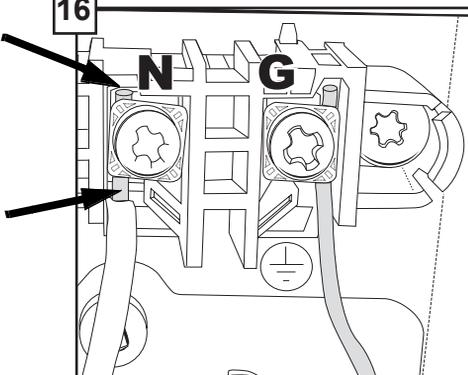
Make sure that the exposed (non-insulated) portion of each stripped wire shows above and below the terminal screw. Securely tighten the terminal screws, but do not **over-tighten** or damage may occur.
