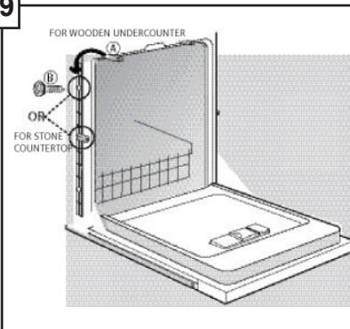
If your countertop is stone, detach mounting brackets (A) from the top and position them at either points on the side. Insert screw (B) through pre-positioned brackets on each side of the unit and attach the brackets.
