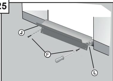
Slide screw (Part F), on the right side first, through the upper hole on the plastic toe panel (Part J), place washer (Part L) on the end of the screw, and attach the toe panel to the dishwasher by tightening the screw. Repeat for the left side.
