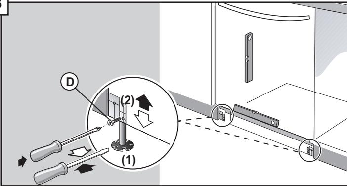
Level the dishwasher horizontally by turning feet (1) clockwise to raise or counter-clockwise to lower front of unit. Once level, (2) insert leg leveler locking screws (Part D) and tighten.
