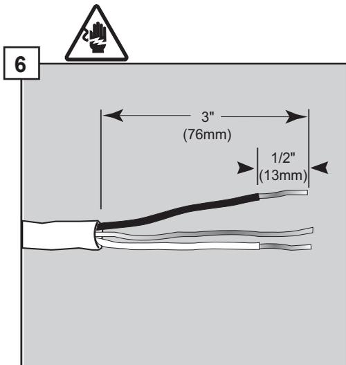
Strip outer casing of electrical wire to expose 3" (76.2 mm) of the inner wires. Then strip 1/2" (12.7 mm) casing from each individual wire.\*
