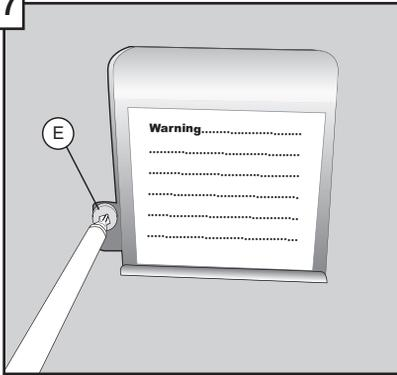
Replace junction box cover. Make sure the cover is seated behind the front lip of the strain relief plate. Attach the cover with the screw (Part E) from the installation kit.
