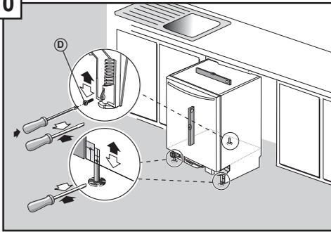
Pre-level unit before positioning under counter by turning feet clockwise to raise or counter-clockwise to lower. Maximum height the unit can be raised with feet fully extended is 34.5" (876.3 mm). Position unit under counter to verify that it is level. If adjustment is needed, remove unit from under counter and adjust as necessary. Once the unit is at a satisfactory height, insert leg leveler locking screw (Part D) in back foot. Step 18 will complete the leveling process.
