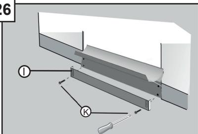
Attach screws (Part K) through the metal toe panel (Part I) to the lower holes of the plastic toe panel so it is flush with the floor. Success! Your installation is now complete.
