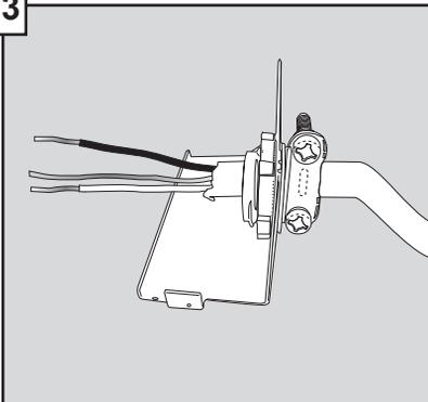
Pass wires through strain relief and plate. Tighten clamp around wires, oriented as shown. Bending the electrical cable as shown will ease installation of the strain relief plate.
