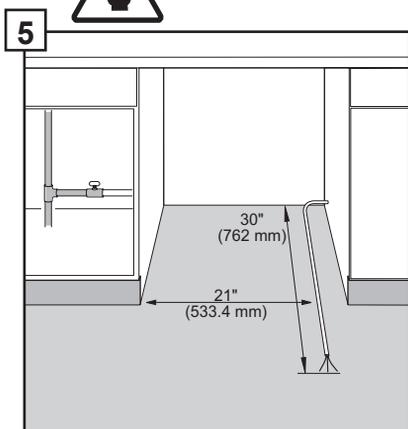
Turn power off at fuse box. Extend cable approximately 21" (533.4 mm) from the opening's left side. Extend the cable 30" (762 mm) from the back wall.
