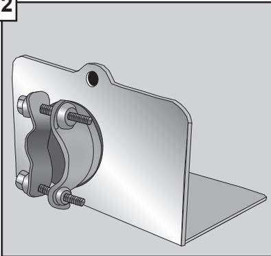
Attach the strain relief (not included) to the strain relief plate. The two screws on the back of the strain relief should be positioned as shown to prevent interferences during assembly. Tighten the strain relief lock nut to prevent the strain relief from turning.
