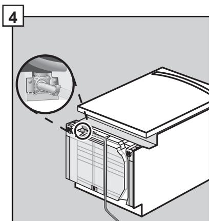
Attach hot water line to 90° elbow and route underneath machine toward hot water connection. Ensure the hose does not contact any moving parts beneath the unit.
