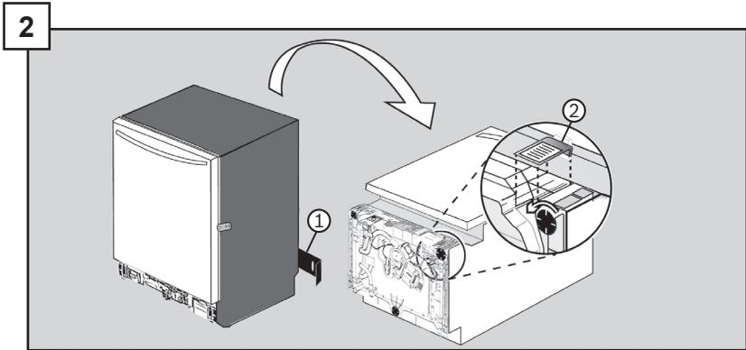
Remove the toe panel(s) (Part H **or** Parts I and J depending on model) (1) from the unit and retain for attachment to the front at a later time. Loosen the leg levelers slightly. Remove junction box cover and retain for later use (2). Discard the small piece of protective styrofoam.
