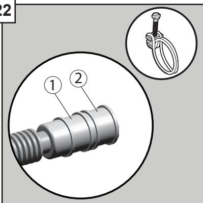
Attach drain hose to plumbing with screw clamp (position 1 for 1/2" [12.7 mm] connection or position 2 for 3/4" [19 mm] connection) and tighten. Do not cut drain hose.
