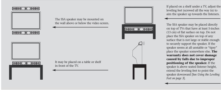
Even if you intend to place the SSA speaker on a TV or shelf you must attach the wall-mount bracket to the speaker. See Using the Leveling Feet on page 3.
