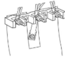
4. Assemble a UL listed conduit connector in the opening.
