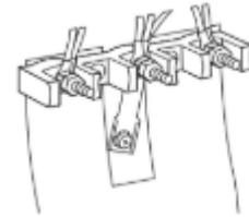
4. Assemble a UL listed strain relief in the opening.
