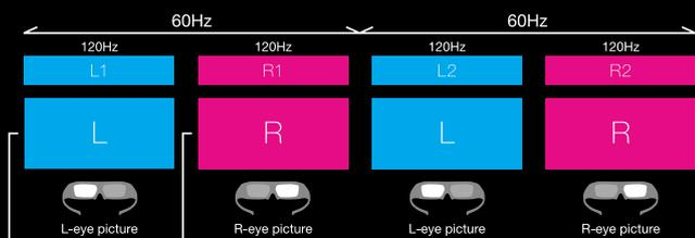
As the shutter can be left open for a longer period, crosstalk is not generated as each frame of the picture is drawn individually without overlap.
