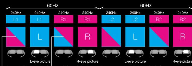
Crosstalk generated where left and right eye pictures overlap during which time, the shutter is closed.
