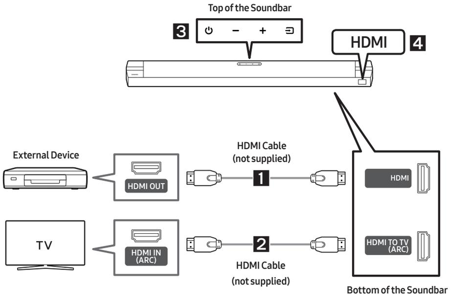
1. Connect an HDMI cable (not supplied) from the **HDMI** port on the bottom of the Soundbar to the HDMI OUT port on your digital device.
