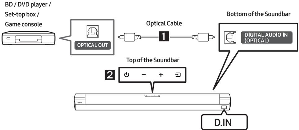
1. Connect **DIGITAL AUDIO IN (OPTICAL)** on the main unit to the **OPTICAL OUT** port of the Source Device using a digital optical cable.
