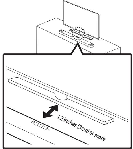
As illustrated in the image, align the center of the Soundbar with the center of the TV, carefully place the Soundbar onto the TV stand.
