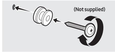
6. Install the 2 **Bracket-Wall Mounts** in the correct orientation on the bottom of the Soundbar using 2 **Screws**.
