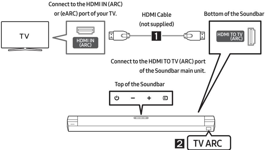
1. With the Soundbar and TV turned on, connect the HDMI cable (not supplied) as shown in the figure.
