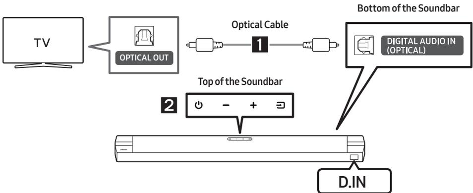
1. Connect the **DIGITAL AUDIO IN (OPTICAL)** port on the Soundbar to the OPTICAL OUT port of the TV with a digital optical cable.
