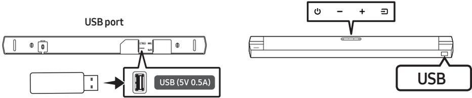
1. Connect the USB device to the USB port on the bottom of the product.
