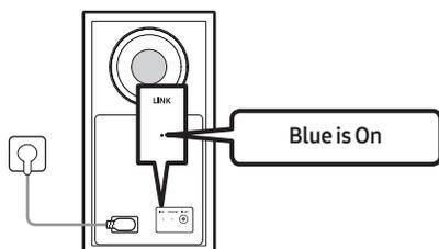
The LINK LED indicator stops blinking and glows a solid blue when a connection is established between the Soundbar and the Wireless Subwoofer.
