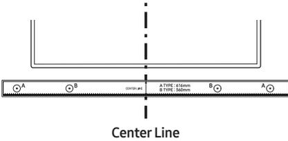
3. Push a pen tip or sharpened pencil tip through the centre of the **A-TYPE** images on each end of the Guide to mark the holes for the supporting screws, and then remove the **Wall Mount Guide**.
