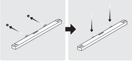
8. Slide the Soundbar down as shown below so that the **Bracket-Wall Mounts** rest securely on the **Holder-Screws**.
