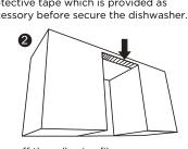
1.Tear off the adhesive film 2.Paste the protective tape on the bottom of counter top. Align the tape to counter edge to better protect from steam 3. Push the dishwasher into the cabinet
