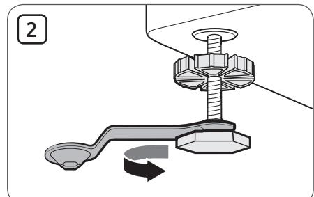
Level the pedestal with a wrench, adjusting all four legs as necessary. Use a level to make sure that the pedestal is level side to side and back to front. Do not tighten the locknuts above the feet at this time.
