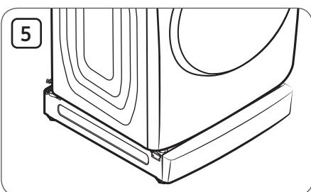
Make sure the legs are tightened before mounting the washer onto the pedestal. Turn the feet of the washer or dryer so that the feet are as close to the body of the washer or dryer as possible, then lock them in place. Place the washer or dryer onto the pedestal so that the feet rest properly in the clamps.
