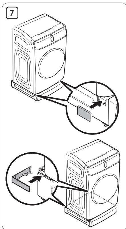
Attach a Guide Cover to each corner of the pedestal. Each Guide Cover is labeled so you can identify the correct corner to attach it to. To attach a Guide Cover, grasp the tab at the corner of the Guide Cover, and then, holding the Guide Cover at a 45 degree angle, slide the 4 prongs (circled on the Guide Cover in the illustration above) under the clamp area, then flatten and push into place.
