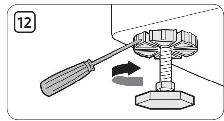
Once the washer is stabilized and does not vibrate, tighten the lock nuts on each leg of the pedestal using a flat head screwdriver.
