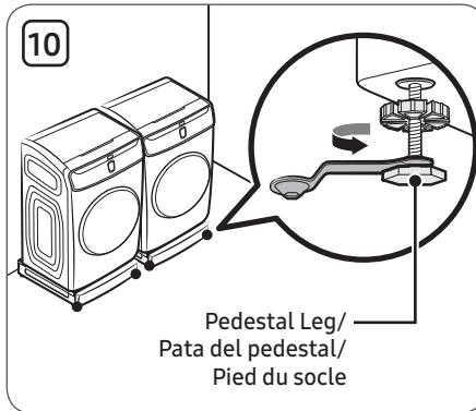
Using a level, make sure the units are level side to side and front to back. Do additional leveling as needed. Proper leveling keeps vibration at a minimum.
