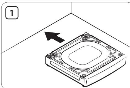
Clean the floor where you intend to install the pedestal, then move the pedestal near where you intend to install it. Make sure to leave yourself space at all four corners so you can access the legs underneath.
