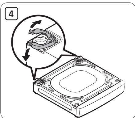
Widen each clamp so you can place the feet of the washer or dryer onto the pedestal properly.
