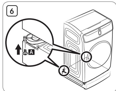
Close and lock the clamps by hand, and then screw Machine Screw (A) through the screw hole of each clamp to secure the washer or dryer to the pedestal.
