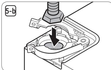
Place the feet of the washer in the outer circle of the safe landing grooves on the pedestal. The location of the safe landing groove for the washer is highlighted above.
