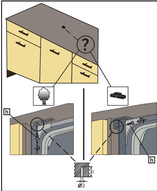
10- Mounting brackets previously fixed to the dishwasher are also fixed in the cabinetry with Screws  $\text{Ø } 5/32'' \times 19/32''$  ( $\text{Ø } 4\text{mm} \times 15\text{mm}$ ).
