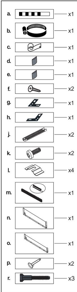
The parts required for positioning the dishwasher are in plastic bags. Check that all of the following parts are contained in plastic bags.
