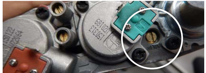
Figure 13.g Adjust pilot size
