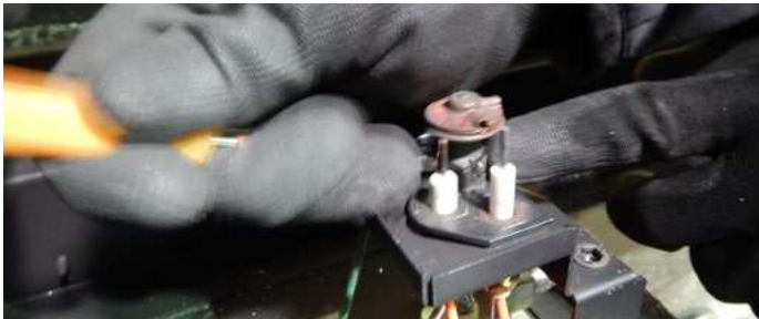
Figure 13.d Removing the spring clip
