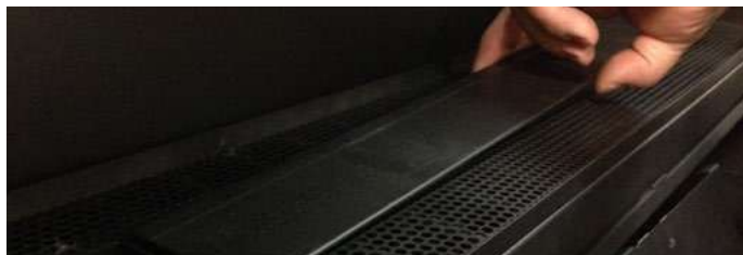
Figure 13.b Loosening the venturi
