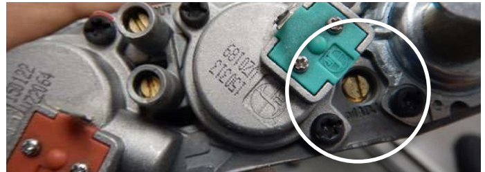
Figure 13.g Adjust pilot size
