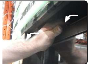
Figure 21.e Lift the door
