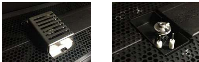
Figure 13. Removal of pilot cover
