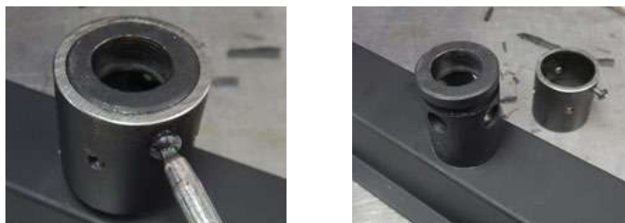
Figure 13.c Removing the orifice
