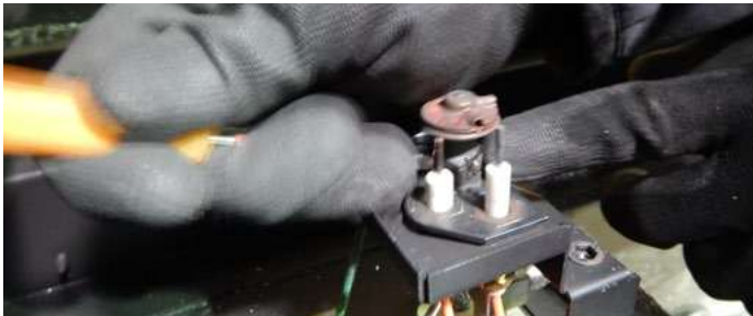
Figure 13.d Removing the spring clip
