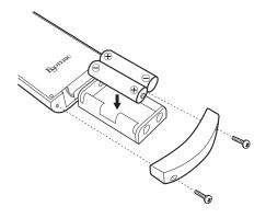
Remove the cover from the back of the remote control and insert two AA batteries with their  $\oplus/\ominus$  ends oriented as shown in the case. Replace the cover.
