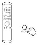
Press the remote control MUTING button to temporarily mute the sound. Press again to restore the previous volume setting.
