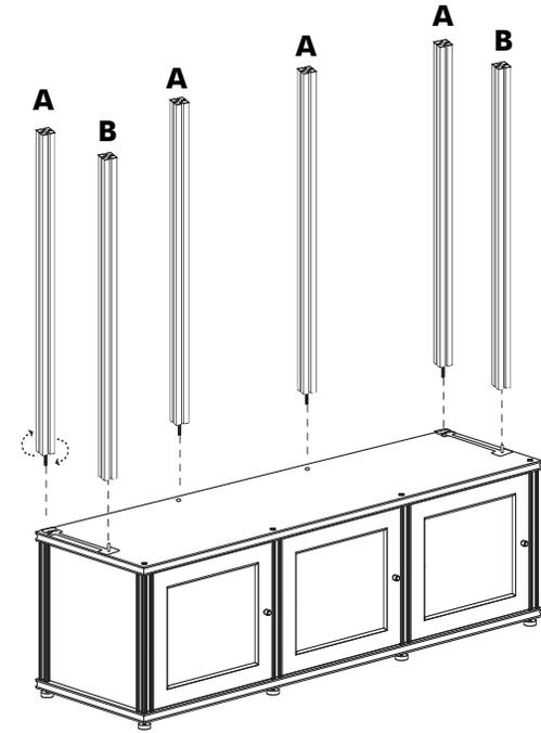
Assemble 2 flat nuts with 2 set screws and slide down the 2 front posts. Place screw through the hole in the post and tighten.
