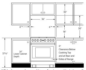
\* Side clearance above cooking surface to any objects, i.e., wall.
