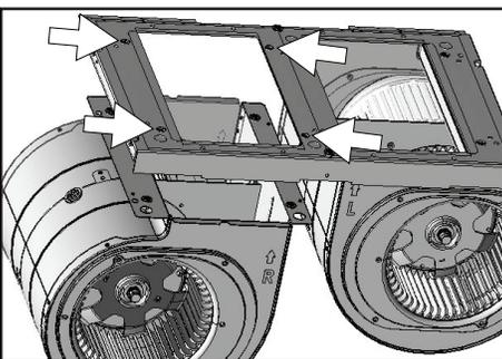
4. Attach single blower to dual blower plate by (4) previously removed screws from step 3.
