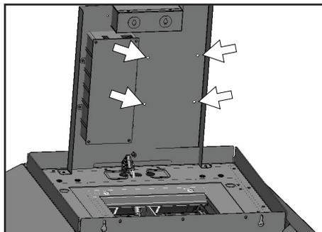
7. Attach dual blower PCB to electronics bracket by (4) screws. Refer to wiring diagram on this step. Connect the wiring from the dual blower including both blower plugs, blower cable 6 pin connector (E), dual blower switch cable (H), black single pin power cord from dual blower (K), and white single pin power cord (F) to dual blower PCB.
