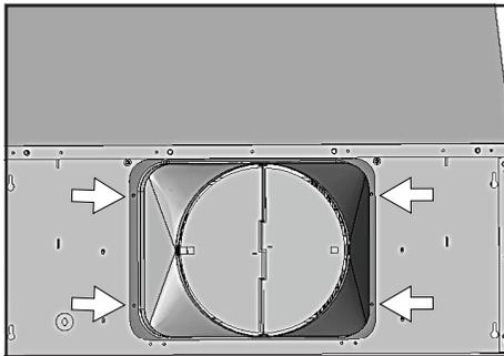
6. Attach 10" round blower collar to top of hood body by (4) M4x8 screws.
