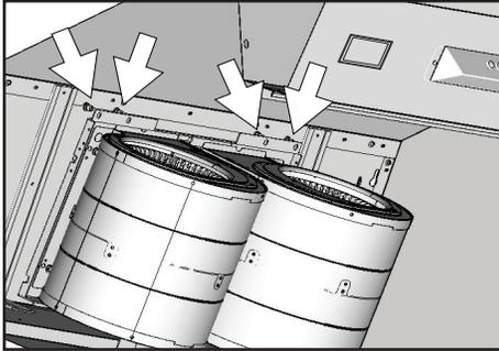
5. Position dual blower inside hood body as shown. Be sure to tuck dual blower plate into blower plate tabs. Secure dual blower by (4) screws previously removed from step 2.
