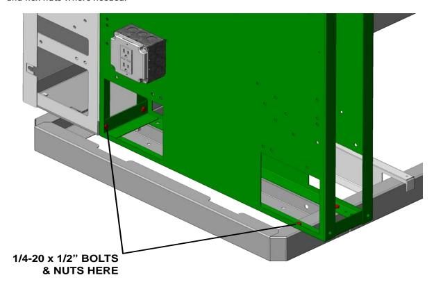
2. Install remaining support walls as you did in step 1. Each wall is numbered and has a corresponding number on the rear wall for ease of locating. (12 foot Outdoor Living Suite with Bar shown).
