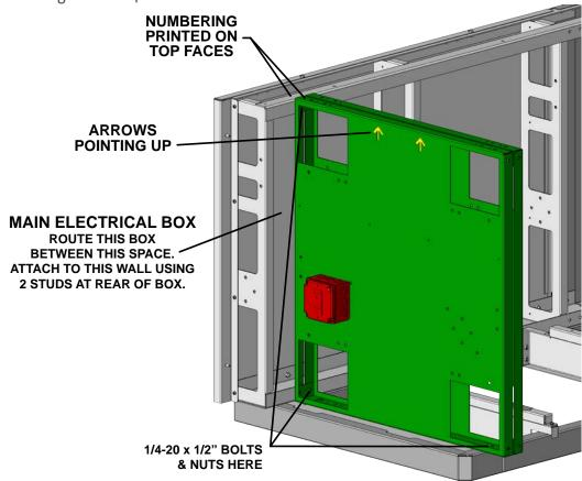
5. Install remaining support walls as you did in step 4. Each wall is numbered and has a corresponding number on the rear wall for ease of locating. (8 foot Outdoor Living Suite shown)
