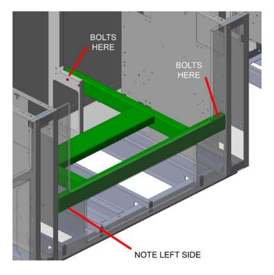
4. The deep alcove for the Kamado Grill may already be bolted to the underside of the large countertop (see below). If the alcove is not mounted, install it first, then the large countertop. Get assistance from another person to help lift the top and position correctly. Install 1/4-20 x 1/2" long hex bolts and flat washers where needed underneath the countertop.
