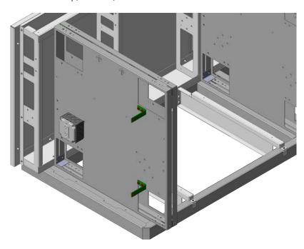
7. Install 2 corner assemblies (4 assemblies for suites with Bar Top). Use 1/4-20 x 1/2" long hex bolts and hex nuts where needed. **Do not tighten until lift-off panels have been checked for proper fit** (see Step 13).
