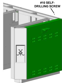
11. Install large front panel as shown using  $1/4-20 \times 1/2''$  long hex bolts and hex nuts located underneath the toe kick area shown below. Also install #8-32 flat-head screws across the top flanges. (8 foot Outdoor Living Suite shown).
