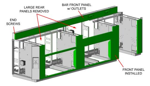
2. The center alcove is shipped loose and must be installed first. Place it in the assembly as shown below. Loosely install three  $1/4-20 \times 1/2''$  long hex bolts and nuts at the rear flange. Do not tighten yet.
