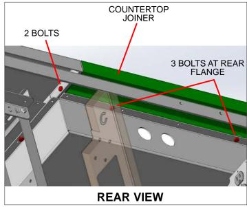
6. Now that the countertops are one assembly, slide everything forward a few inches so you can install the rear panels and center strip as shown. There are bolts across the top, and screws on the ends.
