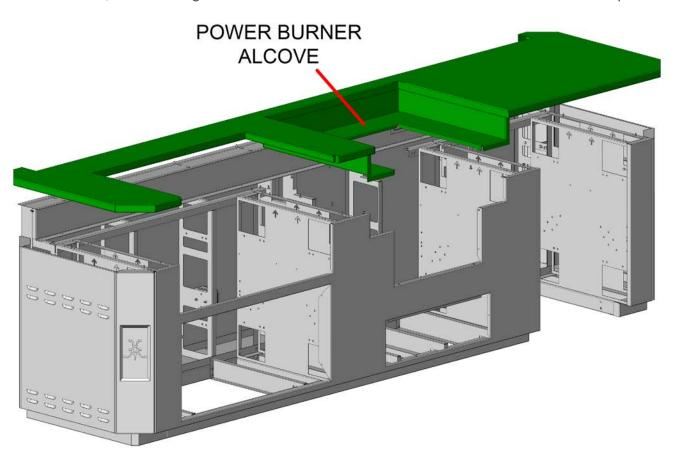
2. There are two (2) #8-32 x 3/8" flathead countersunk screws which attach the alcove to the front panel.
