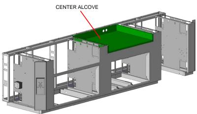
3. Place the left and right countertops roughly in position as shown. There are no fasteners to install yet.
