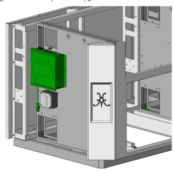
13. Mount the lift-off panel on the left side of the suite. This panel is used to access the electrical box and gas shut-off valve when needed. There are pins on either side for locating the panel. The louvers located on these side panels are needed for ventilation and must not be blocked. If this lift-off panel does not install/remove easily, you may need to adjust the corner assembly(ies) to accommodate (see Step 7).
