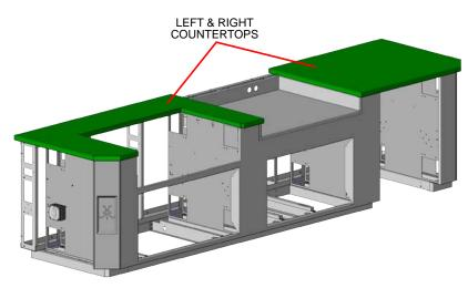
4. The left and right countertops can now be connected to a center countertop joiner. Install 2 bolts on each side of this joiner. Access is from below and the rear. Make sure all 3 top surfaces are flush and flat, and tighten these bolts.
