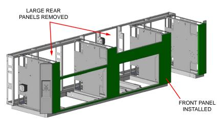
2. The center alcove is shipped loose and must be installed first. Place it in the assembly as shown below. There are no fasteners to install yet.
