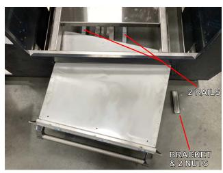
2. With the drawer now fully inserted, reinstall the side bracket you removed in step 1. If necessary, slide out and remove the drawer box so you can gain access to the mounting holes inside the drawer case and secure to those side brackets with four #10 sheetmetal screws (not included). For further details about the drawer box removal and re-installation, see the manual which came with it.
