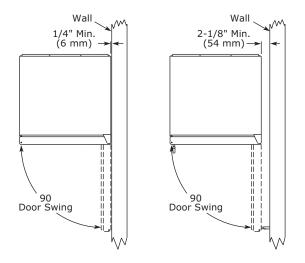
Units have a zero clearance for the door to open  $90^\circ,$  when installed adjacent to cabinets.
