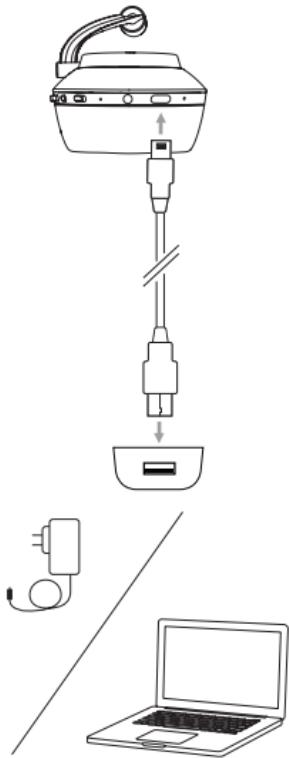
**EN** The indicator on PX will flash green while charging, then turn solid green when fully charged.
