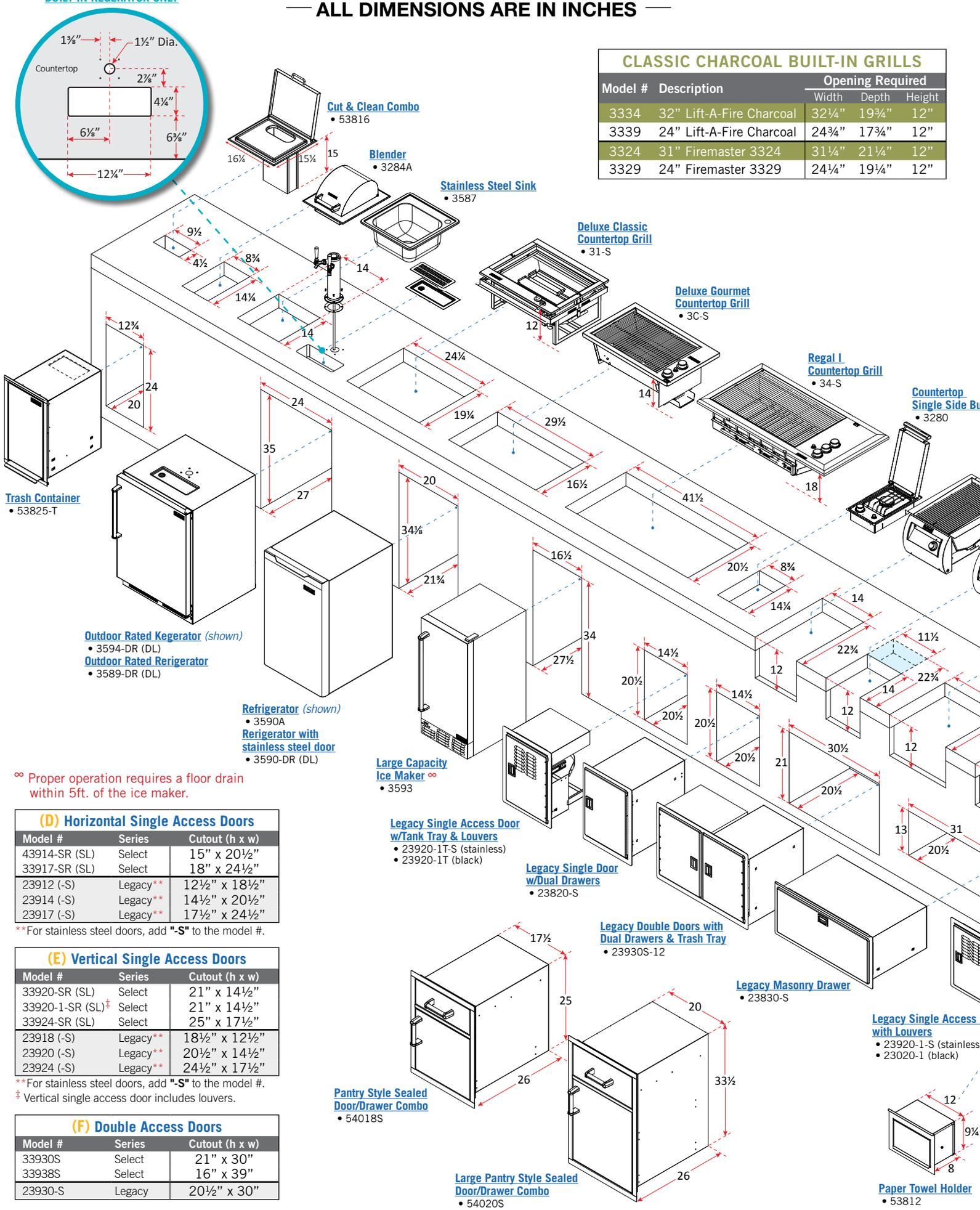
∞ Proper operation requires a floor drain within 5ft. of the ice maker.
