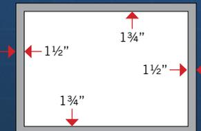
**INSULATING LINER MUST BE USED WHEN INSTALLING IN A COMBUSTIBLE ISLAND**
