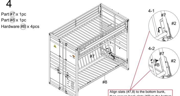
then secure back slats (#7) to the bottom bunk by using bolts (#B).
