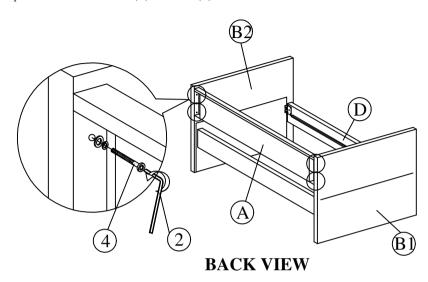
Step 4: Tighten the 4 Corner with Allen Key (1). Install the slats to side rail. Tighten the slats (E) and center rail (K) with CSK screw (8). The distance of the slats should sufficient to obtain desirable bed stability.
