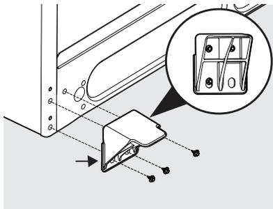
2. Install left toe grille cover onto slot on left side of toe grille.
