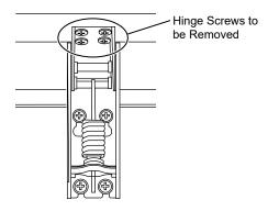
4. To reinstall lid follow steps in reverse. Tighten all hinge screws but avoid over-tightening to prevent stripping. Reinstall hinge covers.
