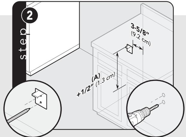
Locate anti-tip bracket on rear wall with the top left corner at measurement (A) plus  $1/2"$  (1.3 cm) from the floor and  $3\text{-}5/8"$  (9.2 cm) from where the right side of range (facing range) is to be located.
