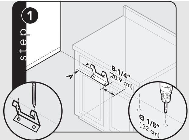
Refer to chart for dimension A based on whether or not standoffs are used with the rear trim device. Mark and drill 1/8" (.32 cm) holes where bracket will be located.
