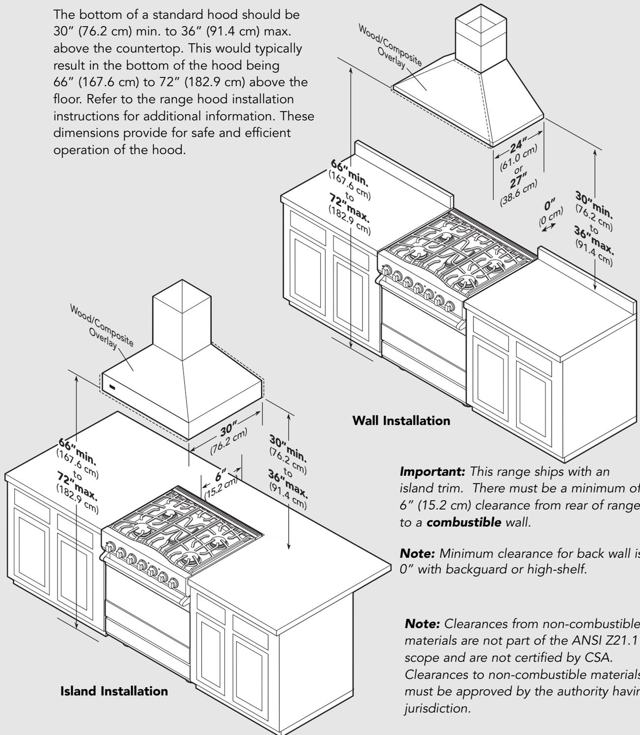
**Important:** This range ships with an island trim. There must be a minimum of 6" (15.2 cm) clearance from rear of range to a **combustible** wall.
