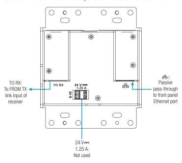
**NOTE:** The 24 Vdc 1.25 A power connector on the transmitter is not used. The transmitter receives power from the included power pack that connects to the receiver only.
