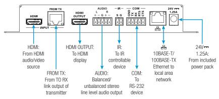
**NOTE:** Only one 24 Vdc power pack (included) is required to power both the receiver and the transmitter. Connect the power pack to the receiver only. Power is transmitted over the cable that connects the FROM TX link input port of the receiver to the TO RX link output port of the transmitter.
